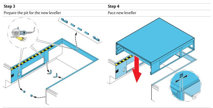
Cut away the rear hinges. Completely disconnect the old leveller's platform from the pit. Keep the old leveller's steel frame in the pit.
